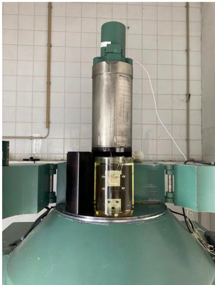
*Exposure of radiochromic films to gamma rays in temperature-controlled water baths.*
